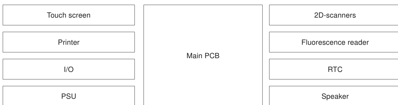
Figure 2.1. Hardware description – Embedded PC with I/O, Power supply unit (PSU), Speaker and Real time clock (RTC), Touch screen, Printer, 2D barcode scanners, Fluorescence reader (opto-electromechanics).
